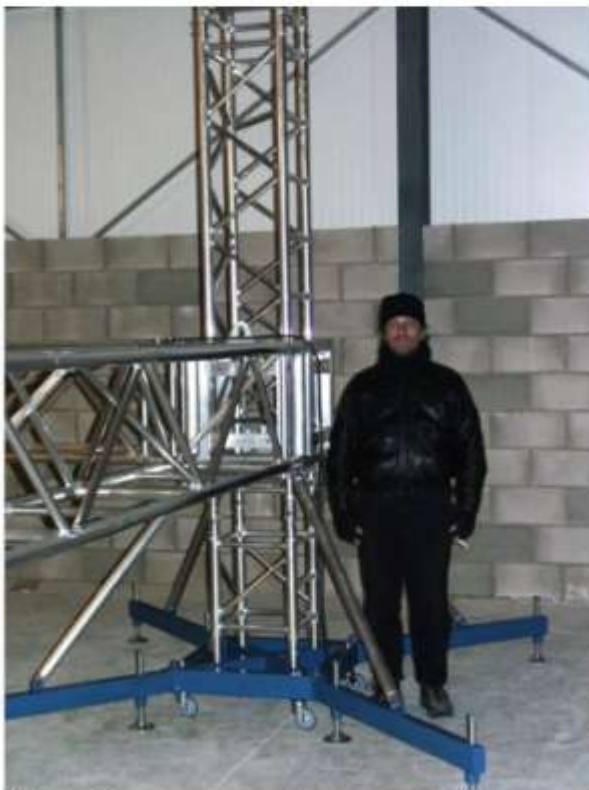
Above: Truss tower outriggers
